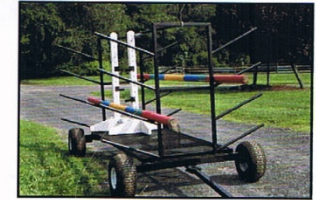
Large Jump Caddy without bed - 4 racks on each side; can carry 64 poles.
